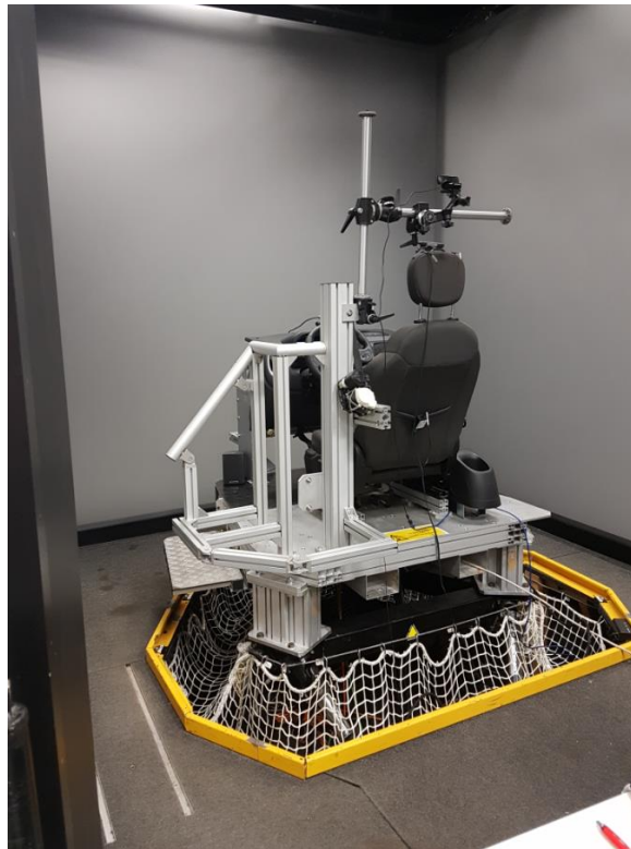
Figure 3.2: Motion platform of CRF driving simulator in Turin
