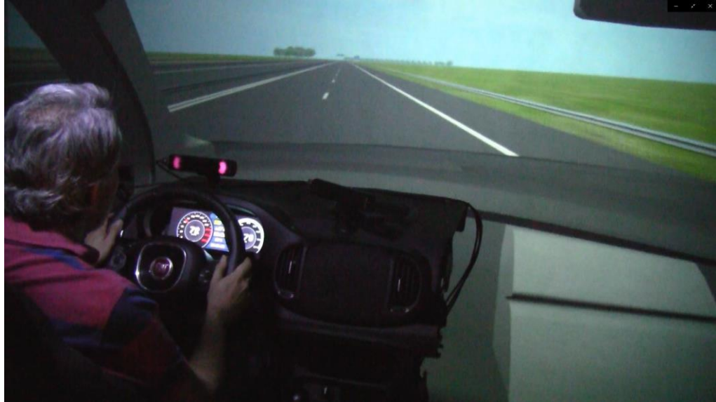
Figure 3.3: Driving simulator with eye detection sensors installed (red lights)
