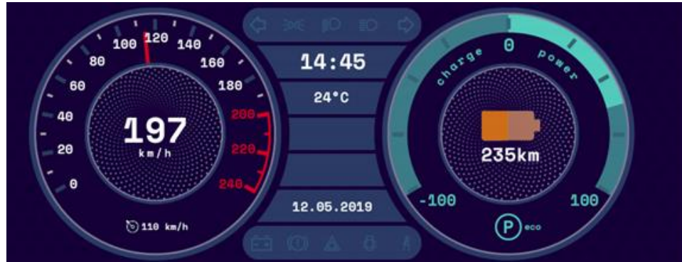
Figure 3.8: The HMI screens showing speed, power and state of charge
