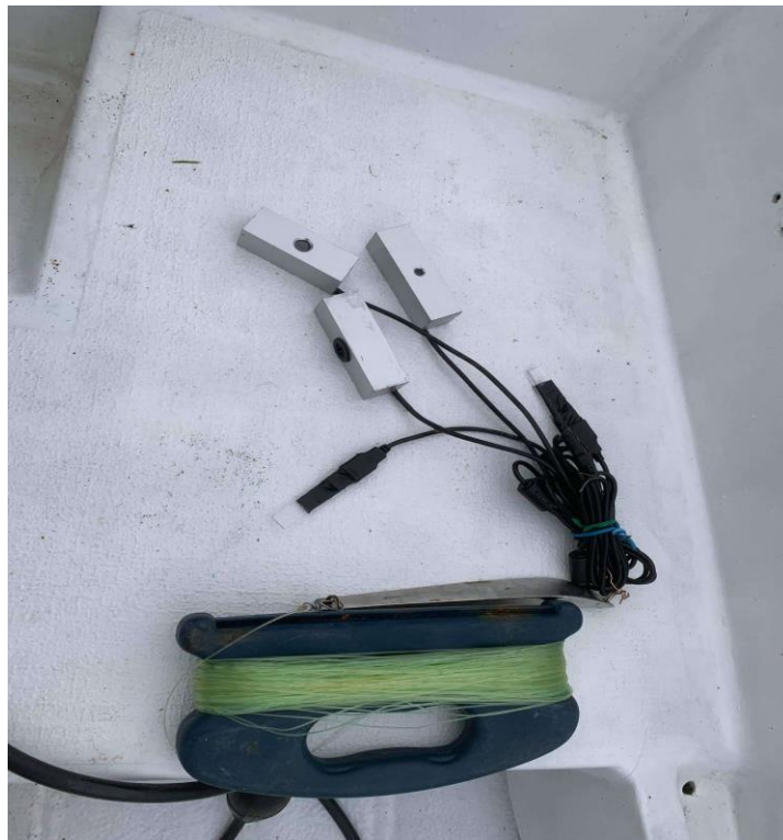
Figure 5.2: the cameras are submerged to different depths with fishing lines in still waters.
