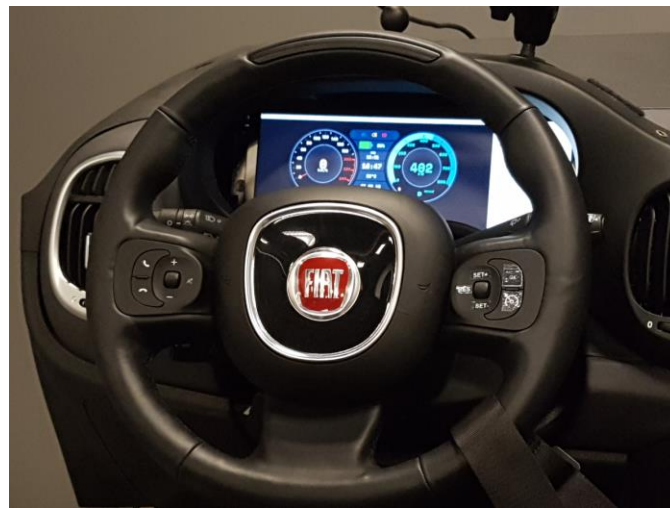
Figure 3.2: One of the two HMI screens showing speed, voltage and state of charge
